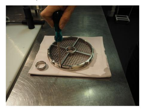
4. Remove the outer locking ring.
