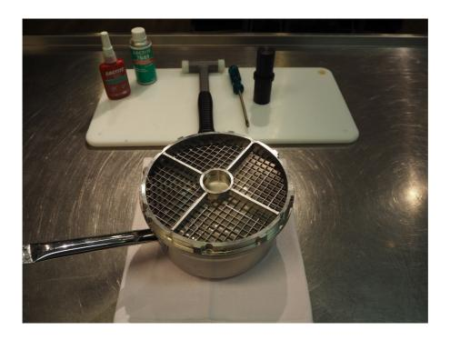
2. Use the HALLDE inner lock ring tool and a mallet to carefully knock lose the inner locking ring.
